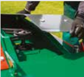
Quarter turn fixings allow quick removal of belt & covers.
