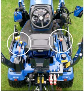
For enhanced safe use of the tractor all controls are colour coded;
