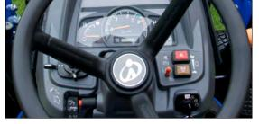
Easy to read electronically operated dashboard with rev counter, fuel gauge, PTO controls and light switches.
