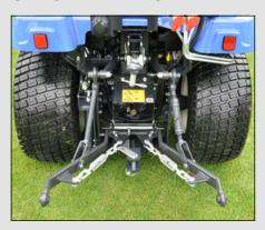
Robust enough to take a variety of implements via a Cat 1 3-point hitch, the controls located to the right-hand side of the seat for ease of operation, the TXGS24 can run a wide variety of implements for a truly versatile machine.
