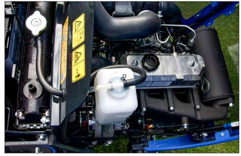
The high torque, powerful and reliable 23hp, 1123cc 3 cylinder diesel engine tackles even the toughest jobs with ease. Its low revving engine at 2,400rpm avoids undue wear and tear on the engine, plus a quieter operating experience.
