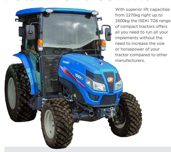
TG6 RANGE • Water-cooled 3 and 4 cylinder diesel engines with displacement of up to 2 434cc
