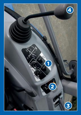
Colour-coded function switches on the left and right operator consoles differentiate the vehicle functions from the hydraulic functions.
