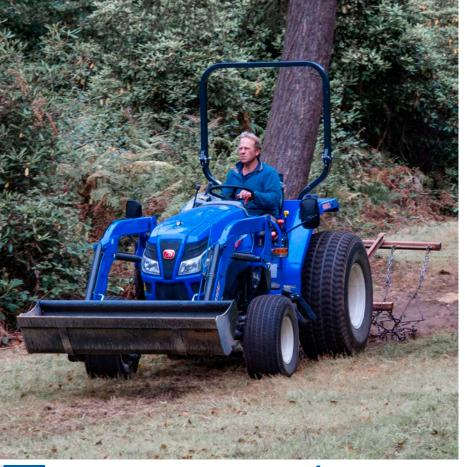
C3 and C4 models are standard whilst the C3+ and C4+ loaders have mechanical self-leveling. All versions have drive-in quick attachments to the tractor for ease of use and quick attachment of implements.
