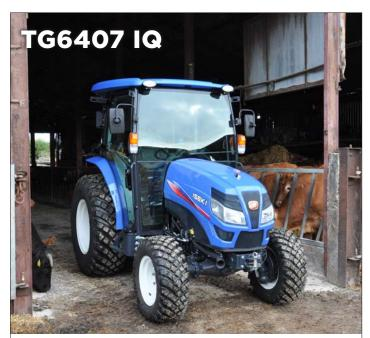
The TG6407 IQ features an ISEKI Stage V, 3 cylinder 40hp diesel engine with IQ Dual-Clutch transmission F24/R24 that offers the control of a manual with the convenience of an automatic. There are 8 clutchless speeds and 3 ranges. Gears are changed by simply moving the gear lever through the straight shift gate. If 'D' is selected then gears 4-8 are operated automatically - ideal for roadwork or
