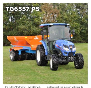
The TG6557 PS tractor is available with a factory fitted, fully air-conditioned category 2 cabin. It features a 55hp four cylinder, Stage V diesel engine, with a F12/R12 power-shuttle transmission.
