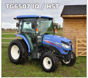
The TG6507 49hp turbo diesel is available with IQ or HST transmission. The HST features the 2-stage servo hydrostat transmission offering three speeds with high and low ranges.
