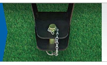
Tow hitch is available to enable you to move a trailer around behind the SXG mower, available whether you have a collector fitted or not.
