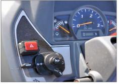
Automotive style dashboard gives clear information whilst operating the mower, plus a fuel gauge to ensure you are never left to accidentally run dry.
