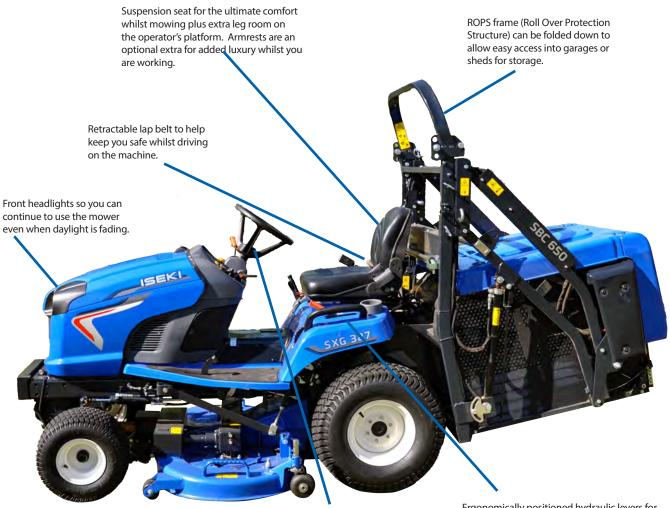
Power steering for easy manoeuvrability whilst out cutting making your job easier and more enjoyable. \*Manual steering only on SXG216+ model. Steering wheel can also be titled and adjusted to ensure the optimum comfort whilst driving.
