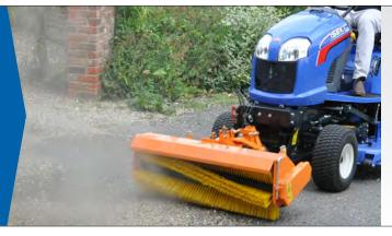
Front PTO comes as standard where you can also add an optional front hitch to carry a rotary brush or snow blade for clearing debris.
