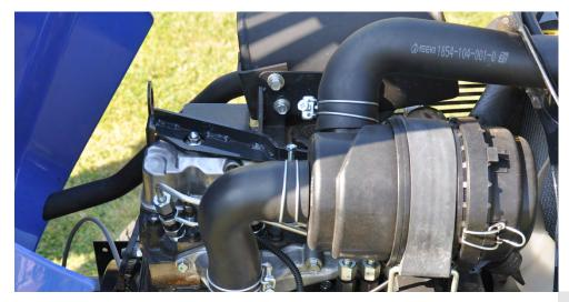
The powerful diesel engine is easy to access for all the daily checks like the dipstick, radiator cover and water with the wide opening bonnet.
