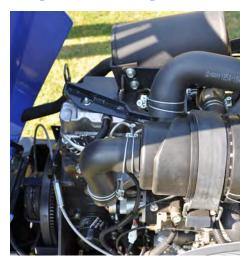
Because of it's large capacity, low revving 1123cc engine the SXG324 and SXG327 creates very little vibration and wear and tear on the engine, whilst also being very fuel efficient and powerful up to 21.6hp. The SXG216+ has a powerful 13.5hp, low revving 688cc, 2 cylinder diesel engine ideal for tackling parks and gardens.
