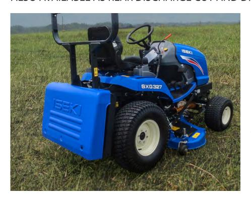
Where grass collection is not required the SXG324 is available as a cut and drop machine utilising a 48" shaft drive rear discharge deck. The SXG327 with its extra power is able to accept the 54" rear discharge deck for more productivity as well as the 48" version. Both decks offer cutting heights from 25mm - 115mm and share the easy cutting height adjustment mechanism found on the rest of the range.
