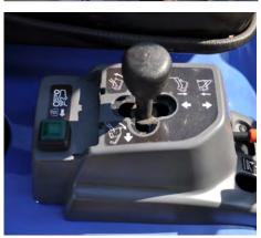
Joy stick control for operating the collector plus a seperate lever for raising and lowering the mower deck. Reverse mow switch enables you to carry on cutting in reverse at the same speed, reducing downtime on turns. It then resets itself when you move forward again.
