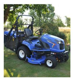
Built to be perfectly balanced, the compact dimensions (2.5-3.3m long) allows the SXG to be incredibly maneuverable, enabling you to effortlessly mow around lawns, flower beds and trees. No extra weights are needed on the front of the machine for stability.
