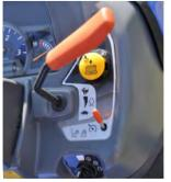
The right hand side of the dashboard now incorporates an electronic PTO engagement switch and cruise control. If the PTO is off and the parking brake on, it is possible to exit the operators platform whilst the engine remains running.
