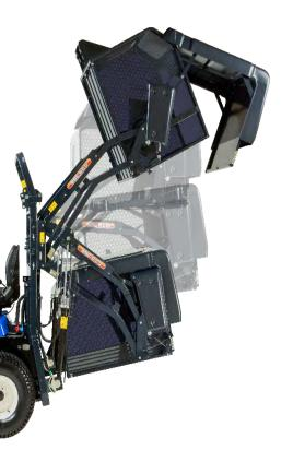
To help make disposing of grass cuttings easy the SXG324 and SXG327 have an hydraulically operated high or low tip collection system which can lift up to a height of 2.08m.
