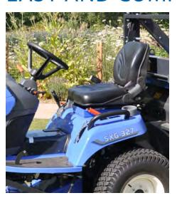
Simple to drive, the 2-pedal hydrostatic system allows for the ultimate control so you can quickly change direction and speed whilst mowing with minimal effort. The large operators platform offers maximum comfort with plenty of leg room, ergonomic controls and suspension seat.
